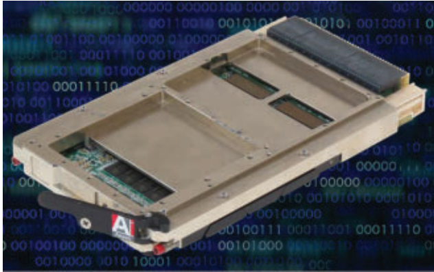
The U-C8500, U-C8501, and U-C8502 3U VPX cyber security-enabled single-board computers from Aitech Systems in Chatsworth, Calif., are aligned to The Open Group Sensor Open Systems Architecture (SOSA) technical standard.
