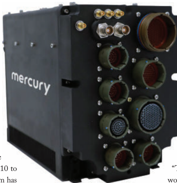
The Avionics Modular Mission Platform (AMMP) 3U OpenVPX avionics mission computer from Mercury Systems Inc. in Andover, Mass., is SOSA aligned and DAL-certifiable.
