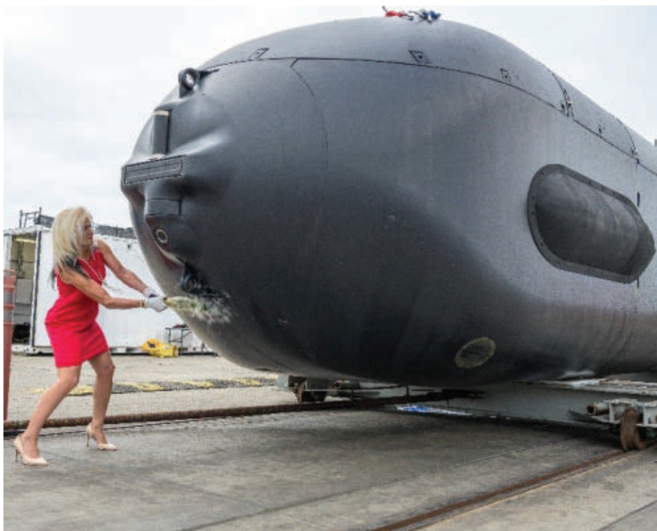
The Boeing Orca XLUUV is an open-architecture reconfigurable unmanned underwater vehicle (UUV) with guidance and control, navigation, autonomy, communications, power distribution, propulsion, and mission sensors.
