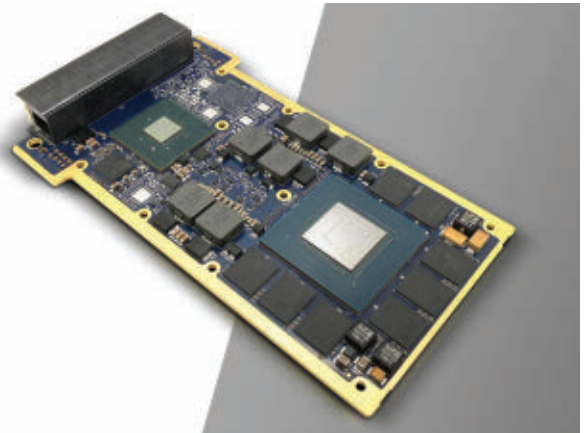
The Curtiss-Wright VPX3-4936 3U OpenVPX GPGPU processor module for artificial intelligence and machine learning is aligned with the CMOSS and SOSA technical standards.
